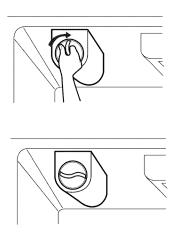
**3.** Flush the water system after replacing filter. Dispense water through the water dispenser for three minutes to flush the system.
